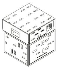
Align the holes with the screws from Step 1 (**Tighten by hand fully**)
